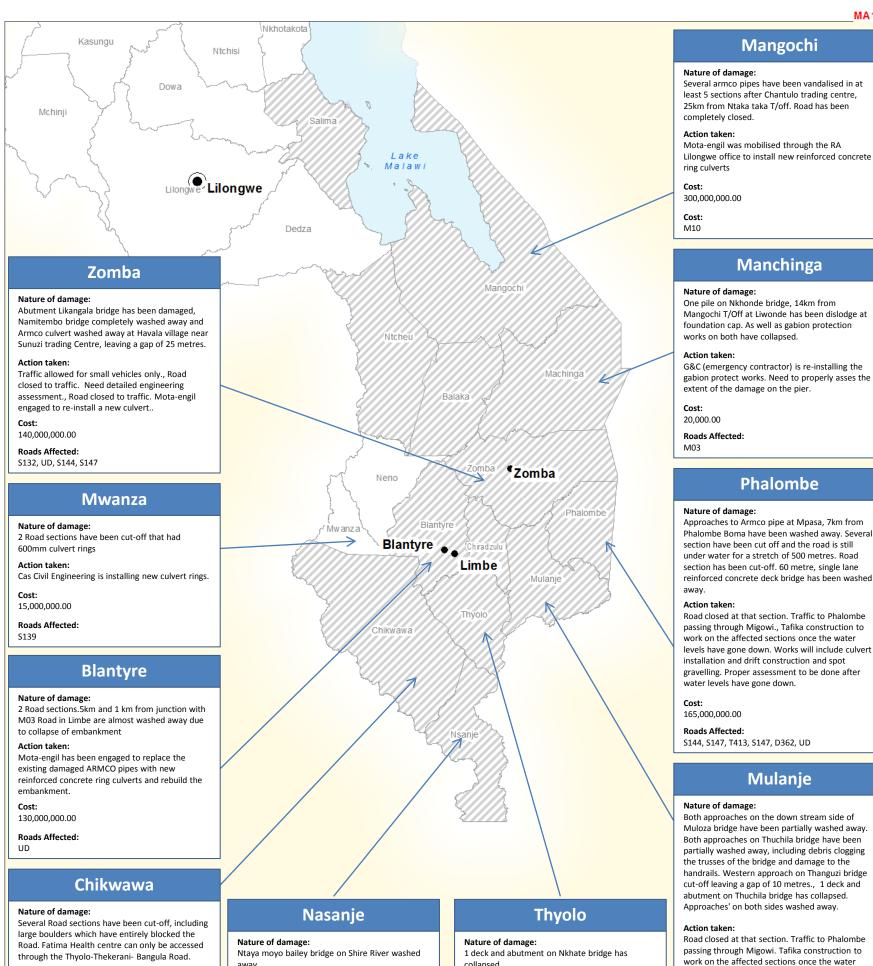
Both approaches on the down stream side of Muloza bridge have been partially washed away. Both approaches on Thuchila bridge have been partially washed away, including debris clogging the trusses of the bridge and damage to the handrails. Western approach on Thanguzi bridge cut-off leaving a gap of 10 metres.,  $\,$  1 deck and abutment on Thuchila bridge has collapsed. Approaches' on both sides washed away
